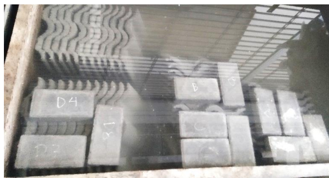
Gambar L-4.3 Proses Perawatan Paving Block
