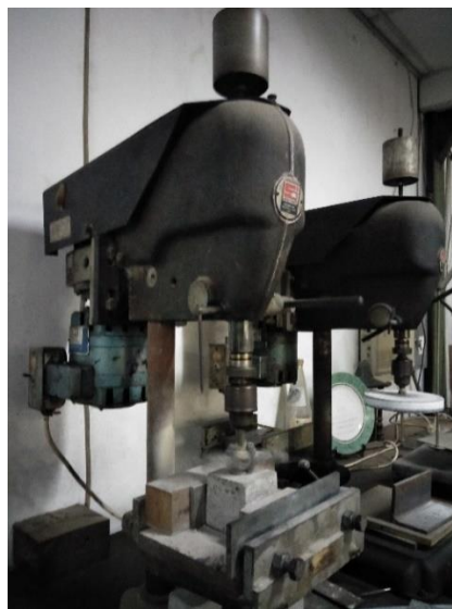
Gambar 5.4 Pengujian Keausan Paving Block
