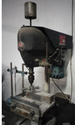
Gambar 4.12 Mesin Uji Keausan Soiltest, INC
