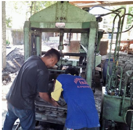
Gambar 4.21 Proses Pencetakan Paving Block
