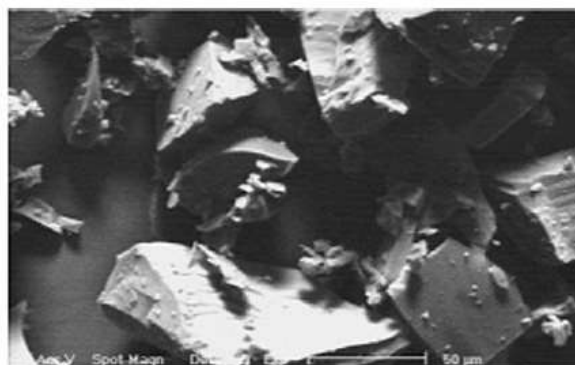
Gambar 3.2 Scanning Electron Microscopy (SEM) filler debu batu
