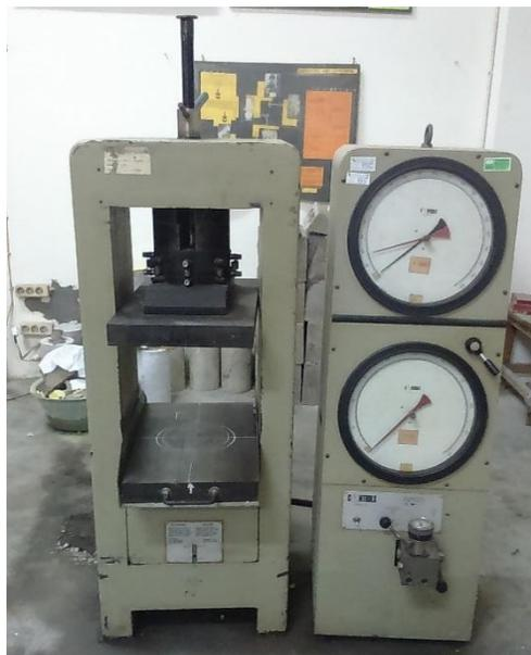
**Gambar 4.20 *Compressing Test Machine (CTM) Merek Control***
