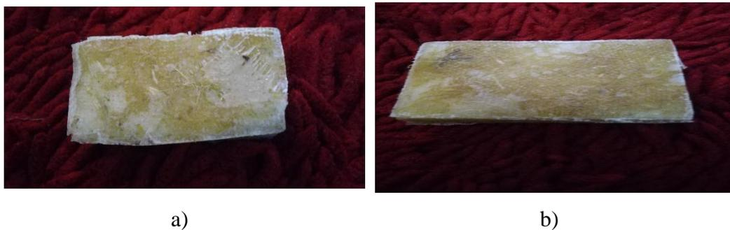
Gambar 4.2 : a) *sandwich handlayup* b) *sandwich vacuum bagging*
