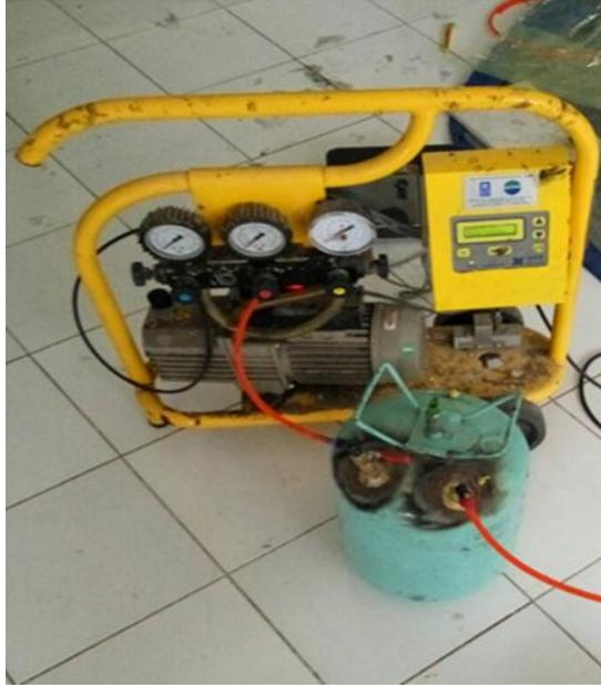
Gambar 3.7 Pompa Vakum
