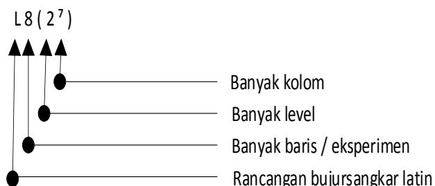
**Gambar 1. Notasi Orthogonal Array**
