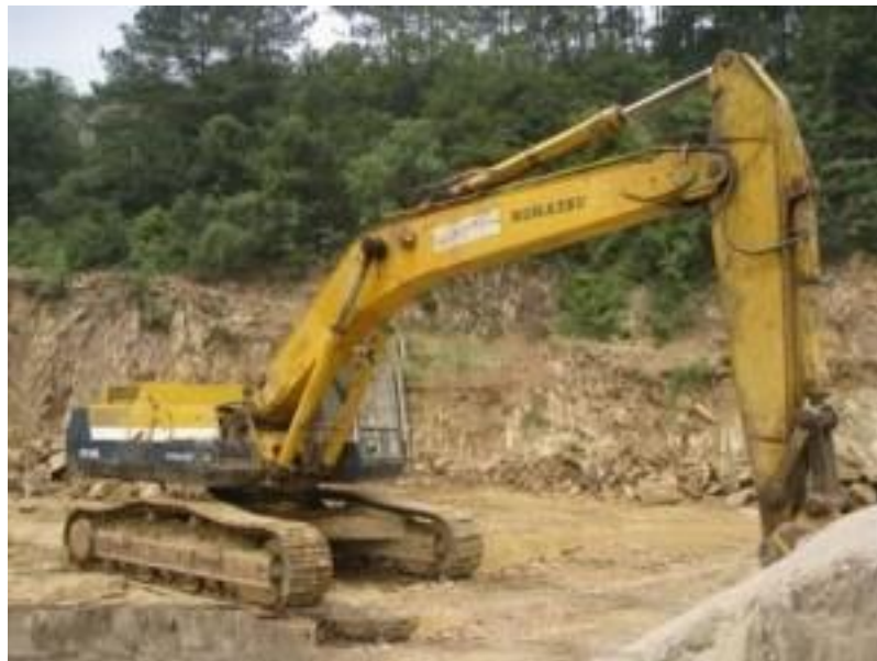
Gambar 3.4 Excavator Komatsu PC400LC-8
