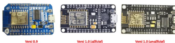
Gambar 2.2 Versi NodeMCU ESP8266
