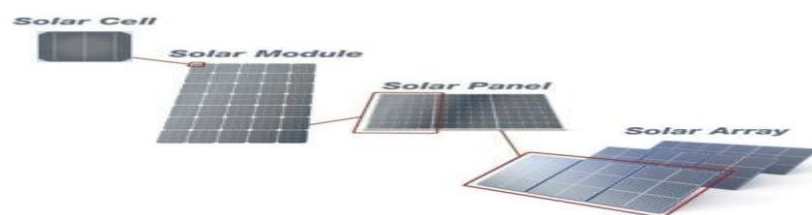
Gambar 2.1 Diagram hubungan sel surya, modul, panel, array[9]
