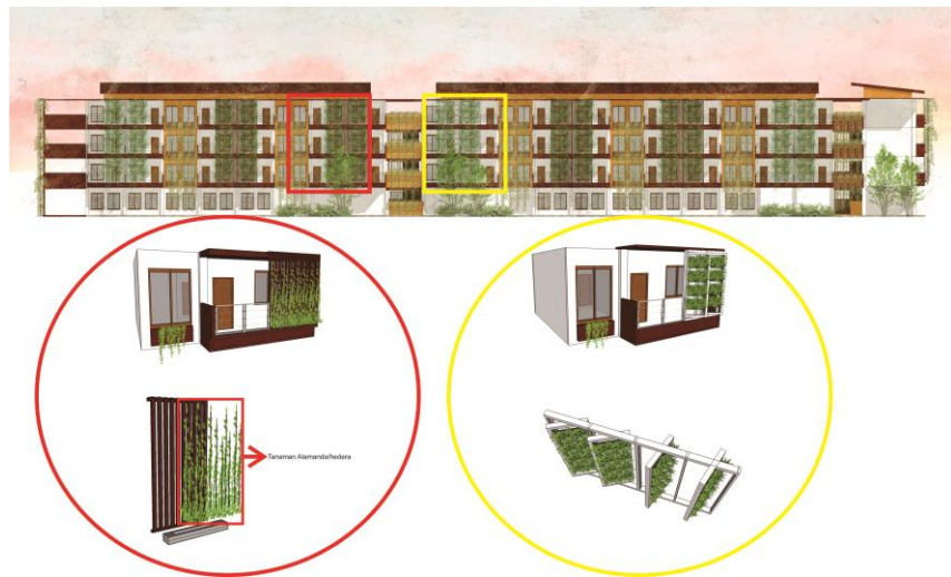
Gambar 5. 6 Detail green facade 2
