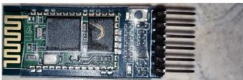
Gambar 2.5 Modul bluetooth HC-05
