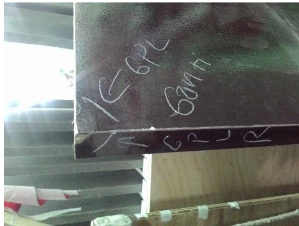
Gambar 4.7 Contoh Jenis Defect Gompal
