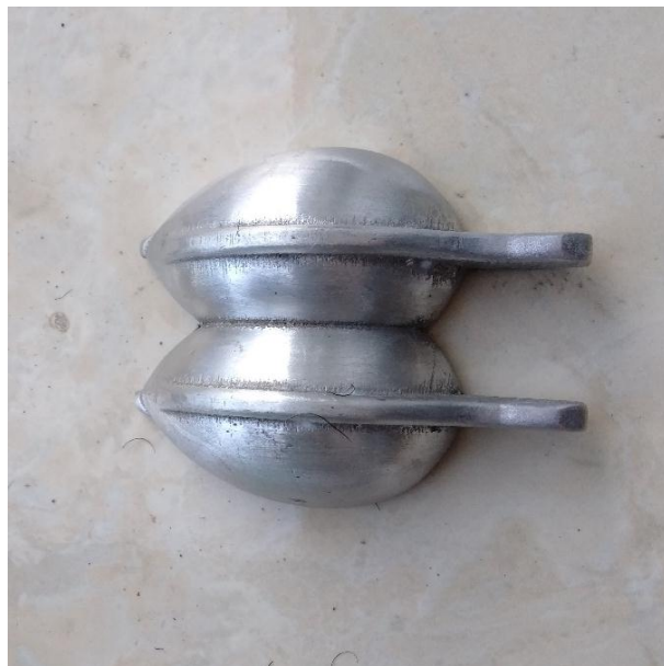
Gambar 4. 9 Sudu Cor Alumunium
