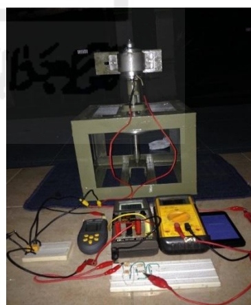
Gambar 11 Rangkaian generator berbeban motor dicouple flywheel
