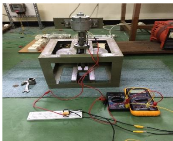
Gambar 7 Rangkaian generator tanpa beban motor tanpa flywheel
