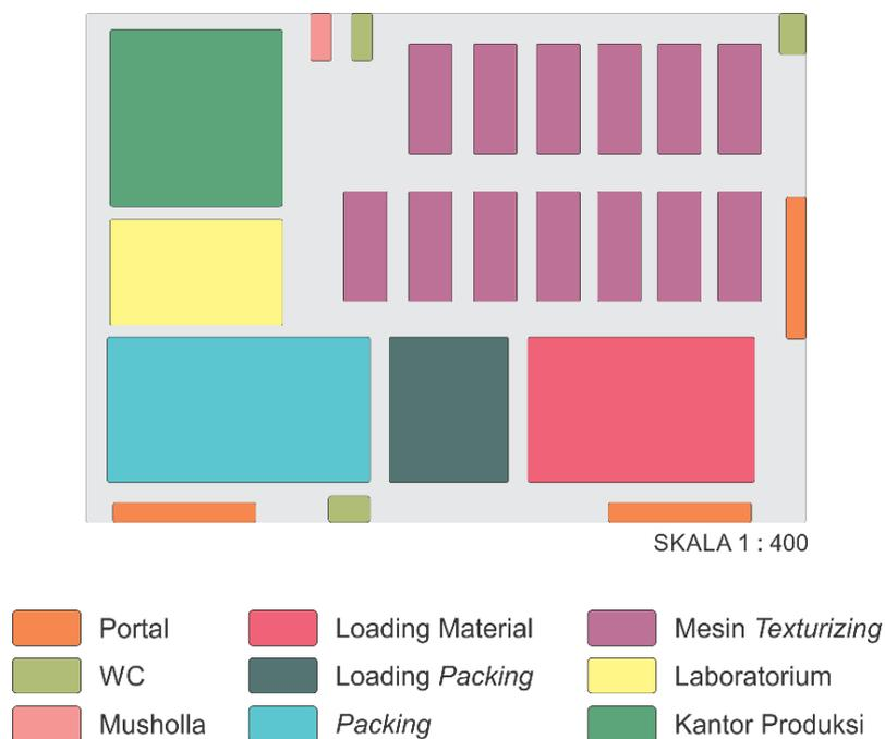
Gambar 4.4 *Layout* Mesin
