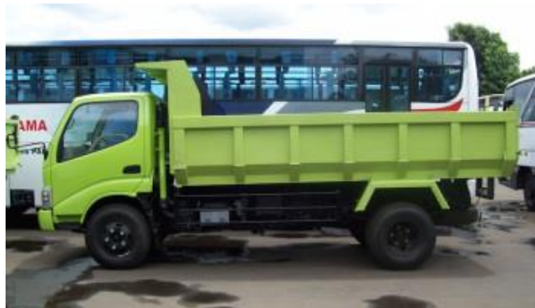
Gambar 3.3 Dump truck kapasitas 7 m 3 (Sumber: www.karoseri.me )
