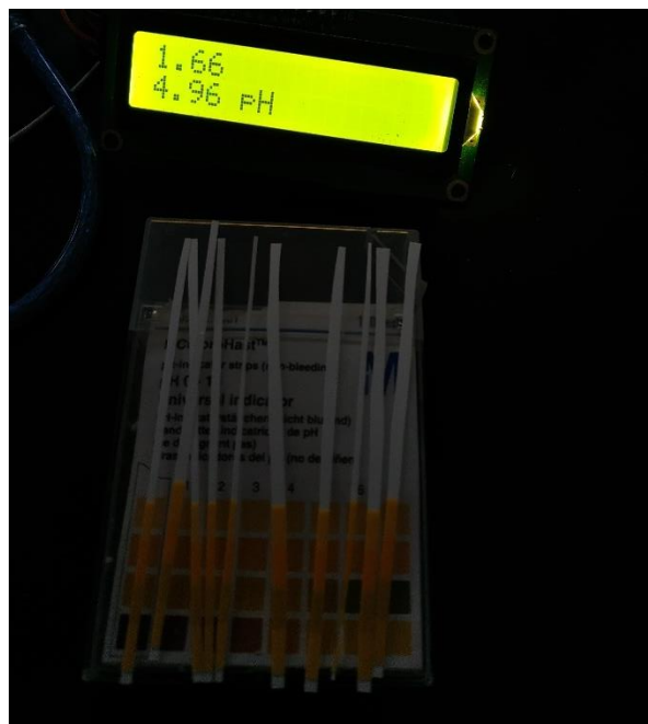
Gambar 2 Proses Pegujian Sensor pH 5
