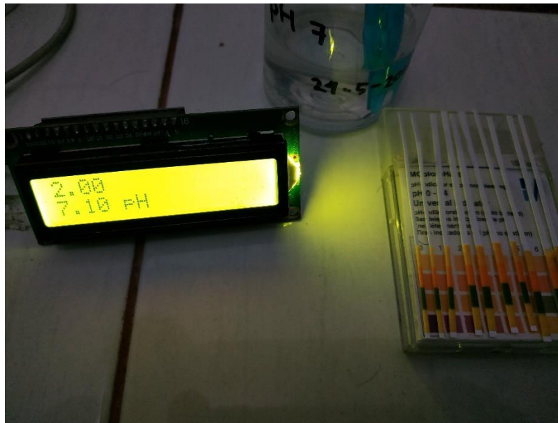
Gambar 3 Proses Pegujian Sensor pH 7
