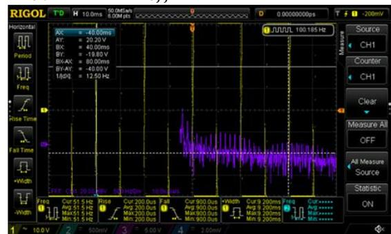
Gambar 12. *Output* beban Lampu 25 W
