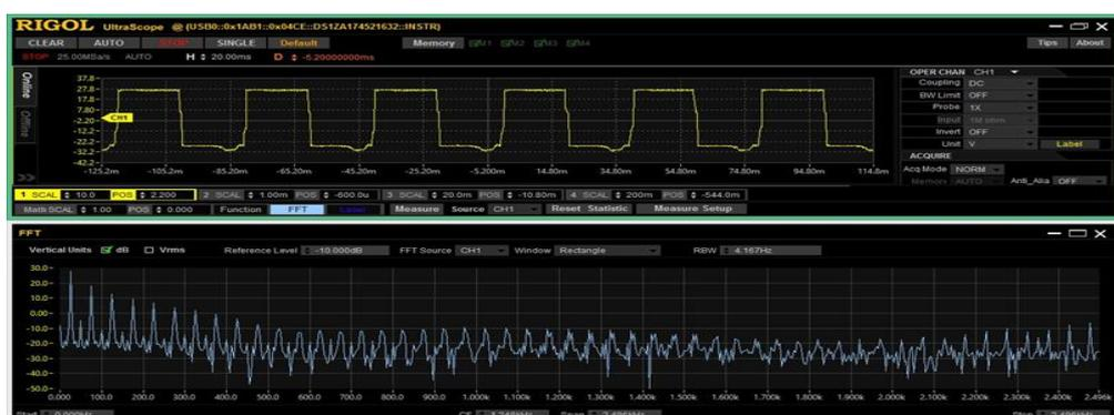
Gambar 3.7 Hasil gelombang *output* inverter 25,99 V
