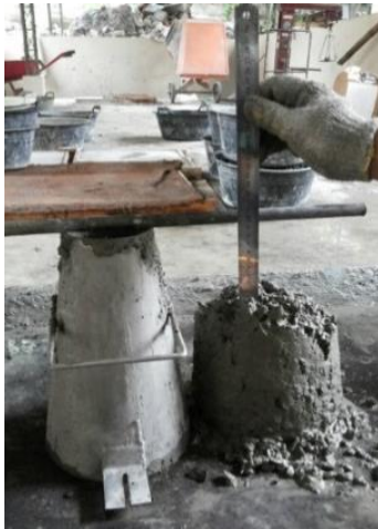
Gambar 7 Slump beton non SCC (BN)
