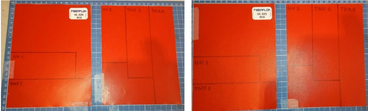
Figure 36 - Silicone rubber coated glass fabric SIL 020 R and SIL 025 R, 15 x 20 cm, 2 pieces of each.
