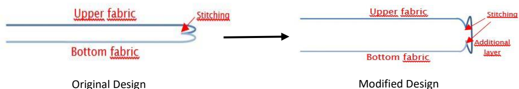
Figure 21 - Modification of original design (1).
