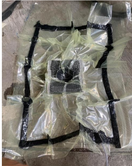
Gambar 3- 42 Vacuum Bagging Produk Puzzle Mold
