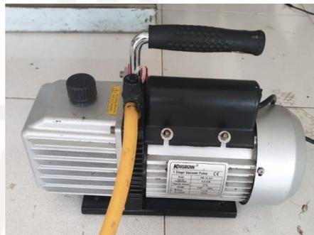
Gambar 3.2 Pompa Vakum
