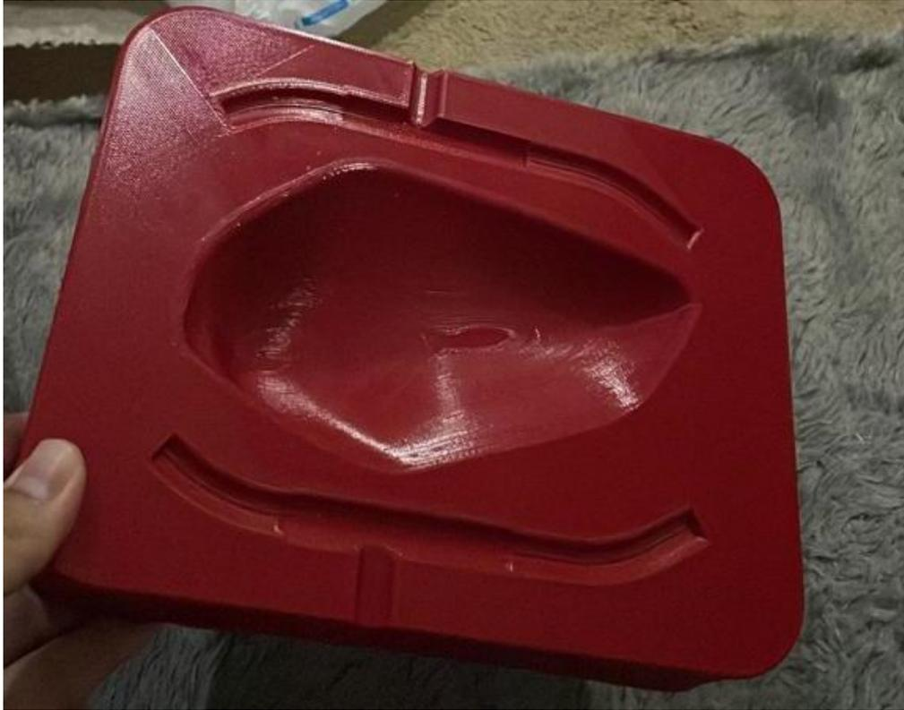
Gambar 4.14 Hasil *3D printing Fused Filament Fabrication (FFF)*
