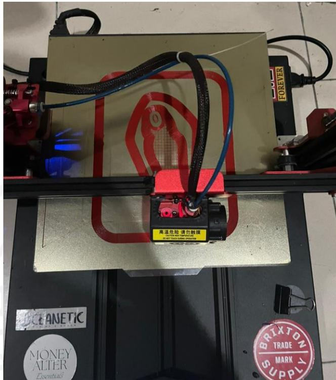
Gambar 4.10 Proses 3D printing *Fused Filament Fabrication* (FFF) 1
