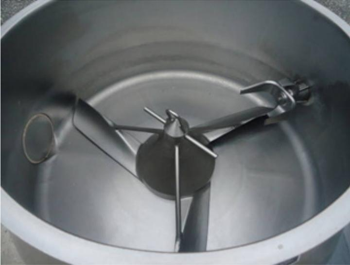
Gambar 5.15 *High-speed mixer/granulator* (sumber: Diosna P 250A)
