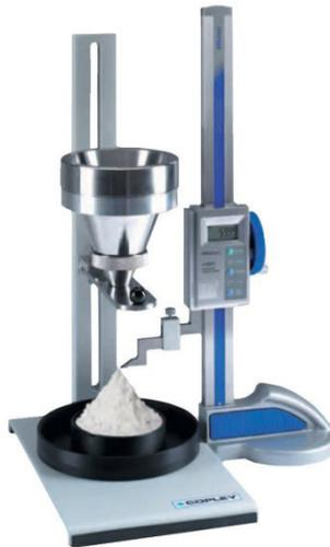
Gambar 2.5 Alat uji sifat alir (*powder flowability BEP2*)(Anonim, n.d.)
