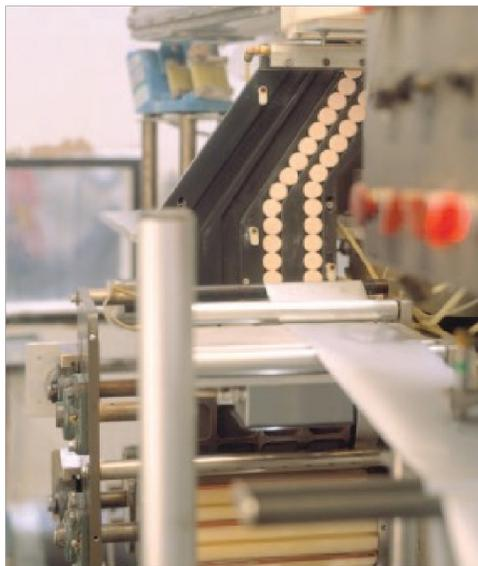
Gambar 7.2 Proses pengemasan tablet effervescent
