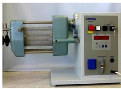
Gambar 5.12 Oscilating Granulator/Erweka-type laboratory oscillatting granulator (sumber: Devay, 2013)
